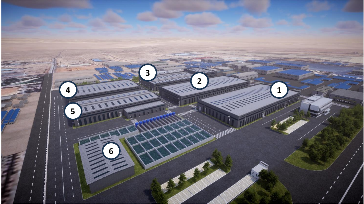
Note: 1. Spheroidization plant; 2. Purification plant; 3. Coating plant; 4. Finishing plant ; 5. Acid storage; 6. Water purification.
