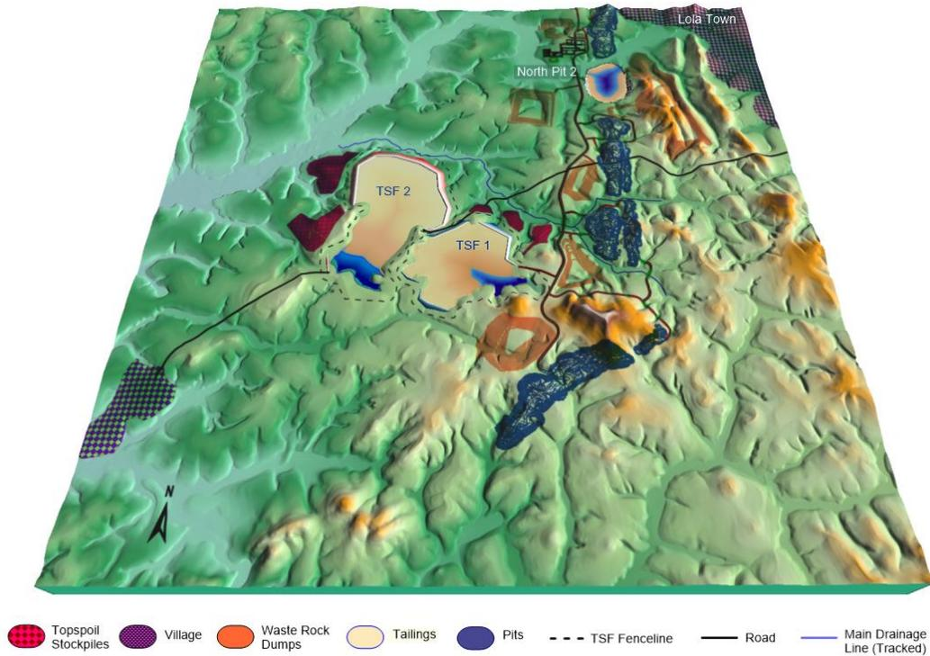
**Figure 18.5 – General Arrangement of the Lola MRDF Site Close Up (2019)**
